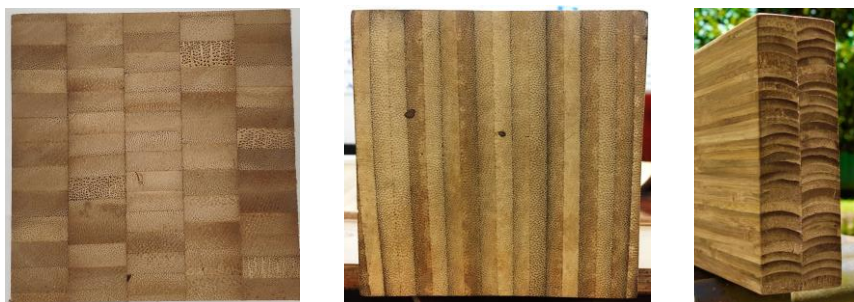
Fig. 2 Cross-sections of three kinds of LBL products
