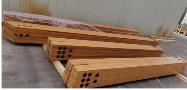
(a) Factory production of LBL sections
