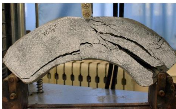
Fig. 5 Failure patterns of cable reinforced arch beam [40]
