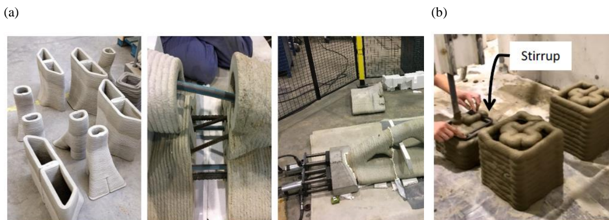
Fig. 1 (a) The Manufacturing process of post-tensioned 3D printed concrete girder [24]; (b) Steel reinforced 3D printed components [25].
