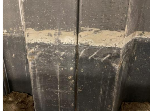
Fig. 32. V-Test 1 sample failure.
