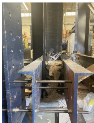
Fig. 18. Increased embedment depth with two channels.
