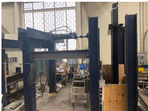
Fig. 5. Sheet pile test set up with Actuator.
