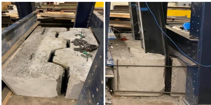
Fig. 16. Restraining structure with elastomeric padding.
