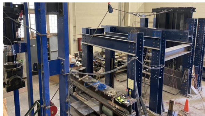
Fig. 6. Sheet pile test set up with Winch.
