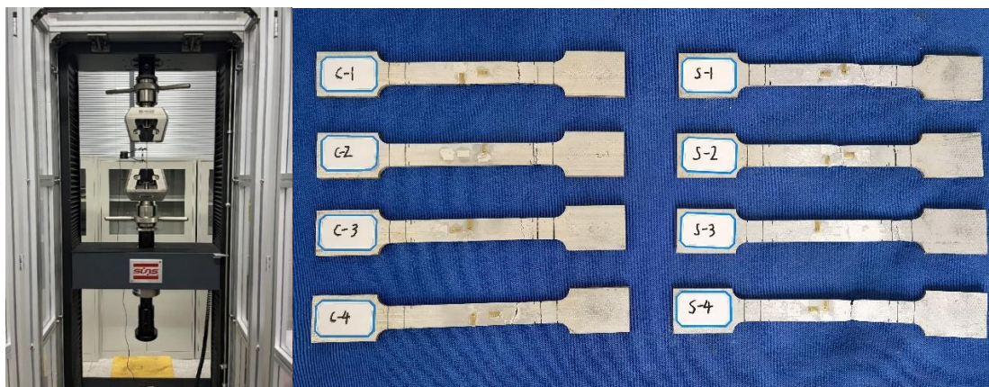
Fig. 7. Test setup and coupons after the tensile test
