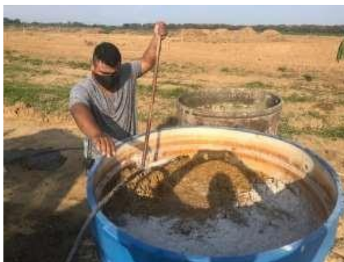
Fig. 9. Mineralization process of rice husk immersed in lime.
