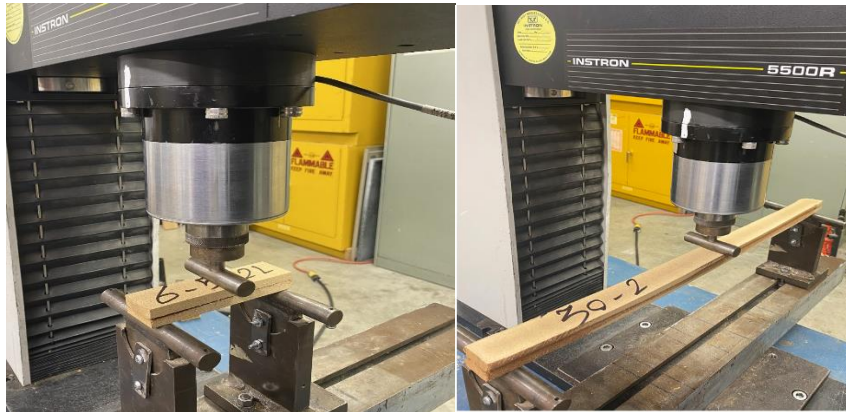
Fig. 1. Center-point loading test of printed timber beams with small span-to-height proportion (left) and large span-to-height proportion (right).
