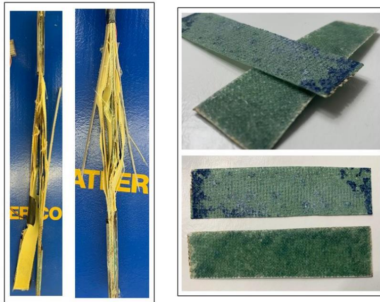
Fig. 16. Failed samples from 8G4KPSVENS (Polystyrene Foam) and removed polystyrene layers.
