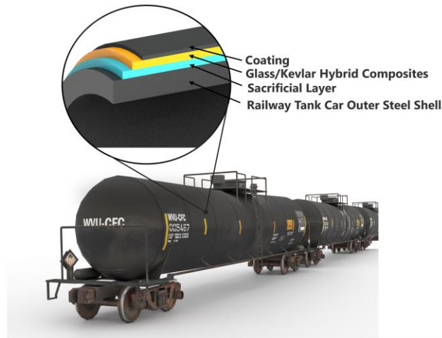
Fig. 1. Proposed FRP composite jacketing for railway tank car.
