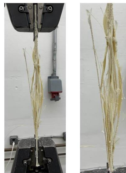
Fig. 10. The failure mode of 8G4KNCVENS samples under tension
