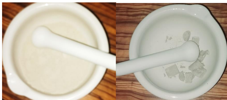
Fig. 5. Grinding of hardened clay-lime paste sample
