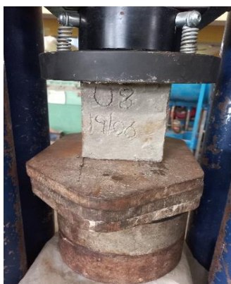
Fig. 4. Strength test on mortar samples
