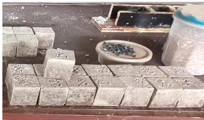
Fig. 2. Mortar sample cubes (50x50x50 mm)
