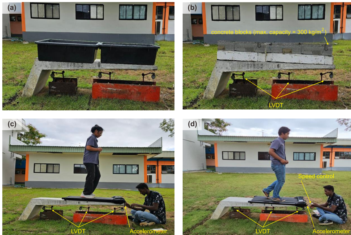
Fig. 7. Test setup and instrumentation of: (a) short-term flexural tests, (b) long-term flexural tests, (c) female and (d) male walking scenarios.
