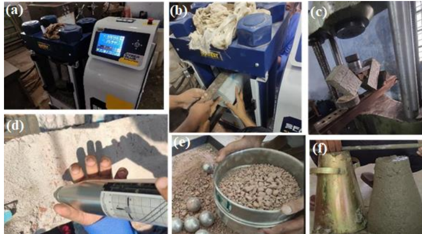
Fig. 4. Tests of RBAs and ReC made with them.
