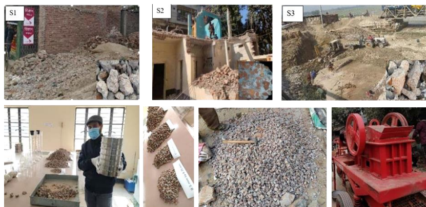
Fig. 1. Collection of concrete blocks and processing them to RBA.
