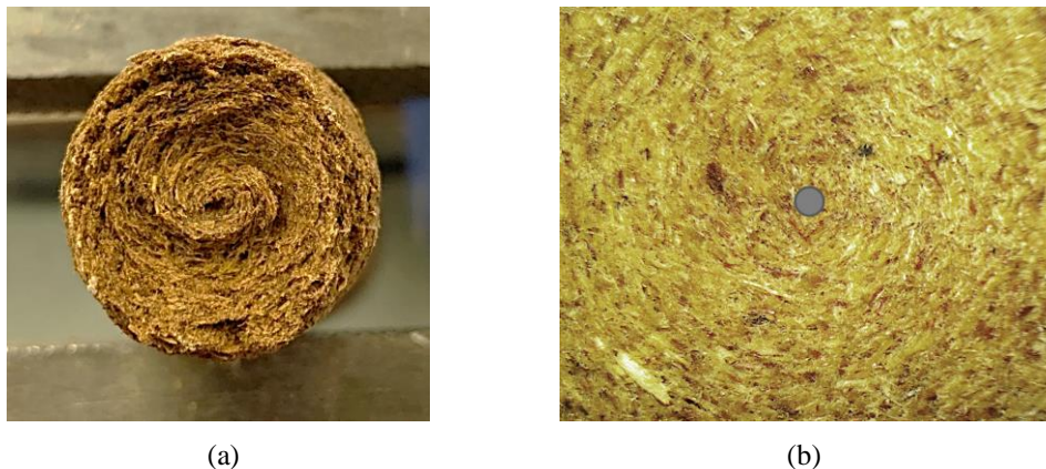
Fig. 9. (a) Cross-sectional view of the highly compressed wood-sodium silicate mixture upon extrusion from the nozzle. (b) Magnified optical micrograph of cross section of the extrudate exiting from the nozzle with the center denoted by the gray circle.
