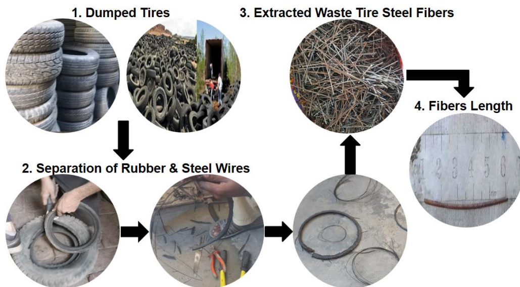
Fig. 1. Process of extraction of steel fibers from waste tires
