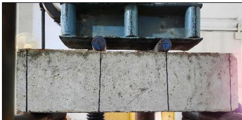
Fig. 7. Three point loading arrangement
