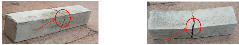
b) Non-separation of the sample(with fiber) c) Separation of the sample(without fiber)
