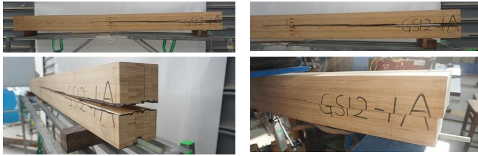
Fig. 6 End shear failure
