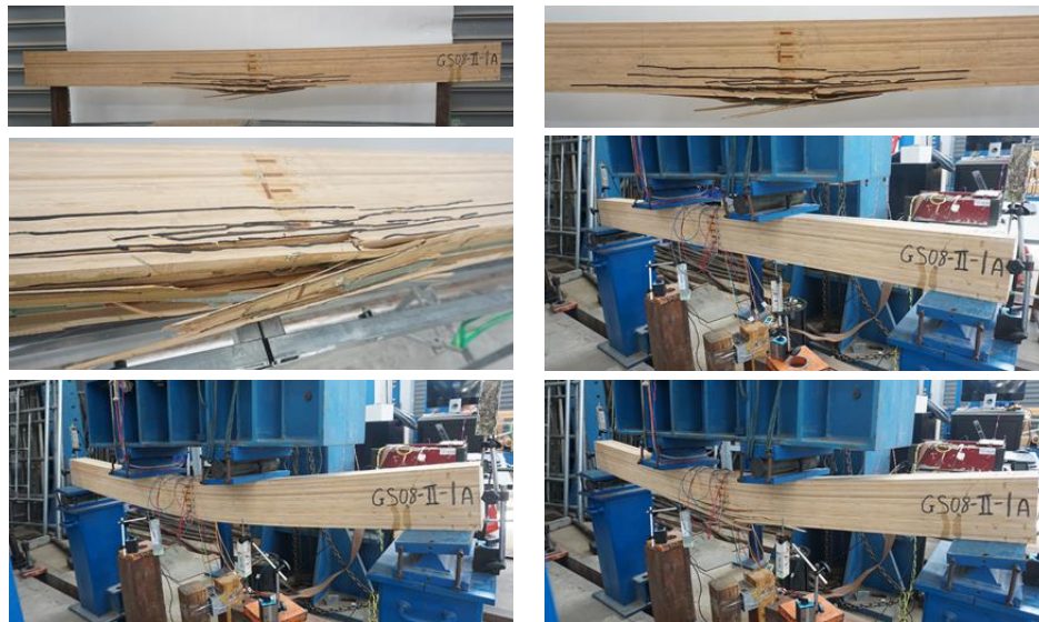
Fig. 5 Fracture of bamboo fiber in the tension zone
