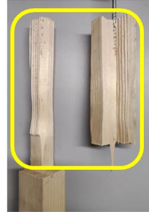
**Fig. 9(c).** Shear fractured piece.
