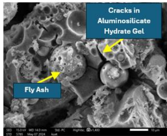
Fig. 14. SEM analysis after thermal exposure @200 °C
