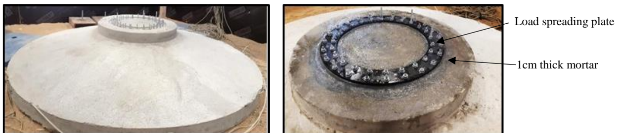
Fig. 11. Implementation of 1/10 scale reinforced concrete footing; a) 20 days after casting and b) mortar casting under load spreading plate
