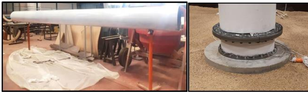
Fig. 12. Superstructure of the 1/10 scale model; a) Before placement and b) after connection to the footing through a bolted system.
