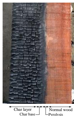
Fig.1. Charred sample showing charred layer, pyrolysis and normal wood
