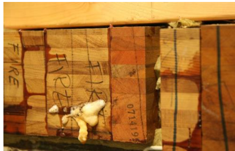
Fig.9. Moisture evaporation and foam on the surface of the charring test specimen B (fire-retardant treated)
