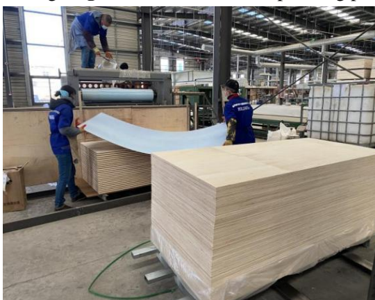
Fig.3. LVS-laminated facing assembly
