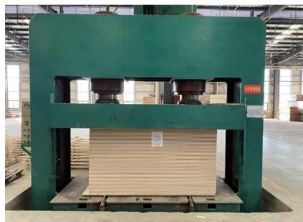
Fig.4. Cold pressing of LVS plate
