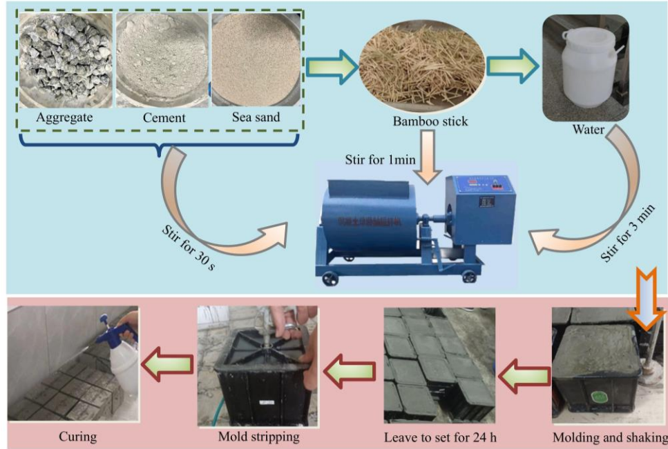
Fig. 4. The main process of preparing BFRSSC.
