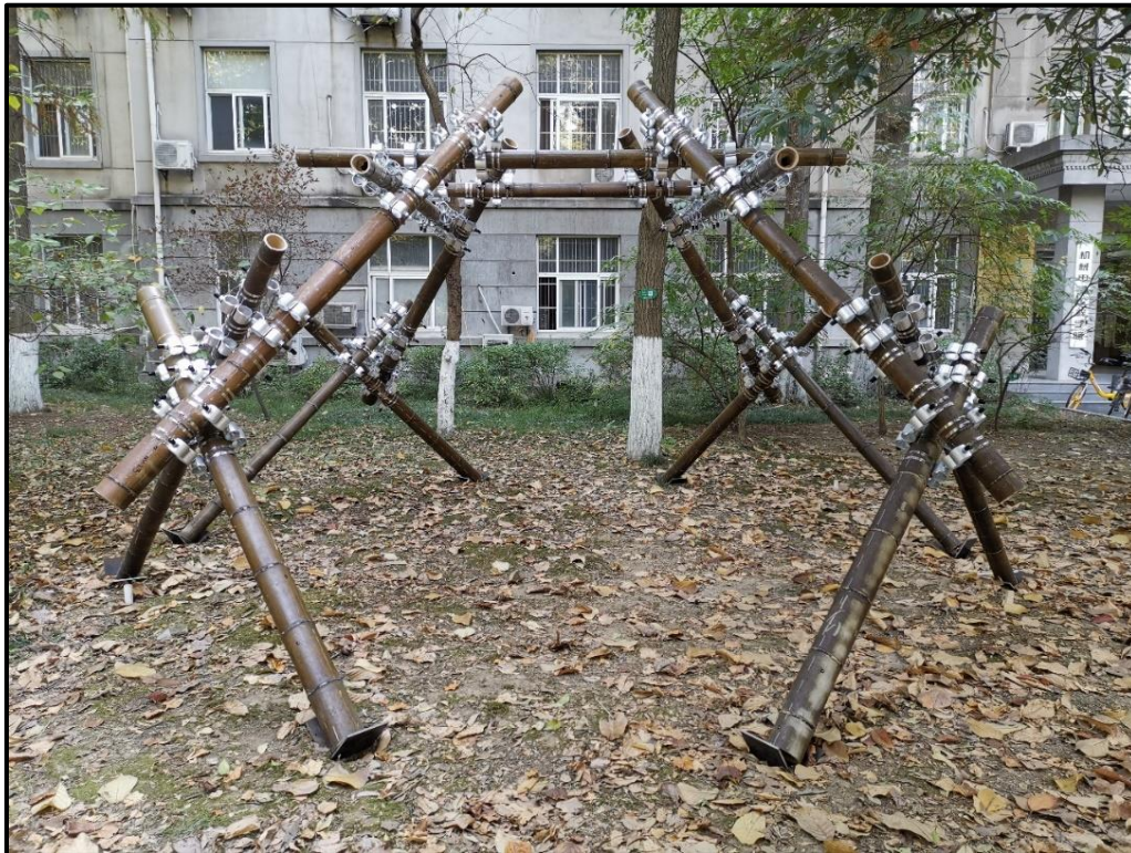
Fig. 11. Modular Bamboo Space-Frame Structure with Metallic Connectors
