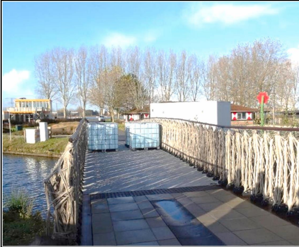
Fig. 9. Static test with four barrels in the center (reproduced under the creative commons attribution license) [160]
