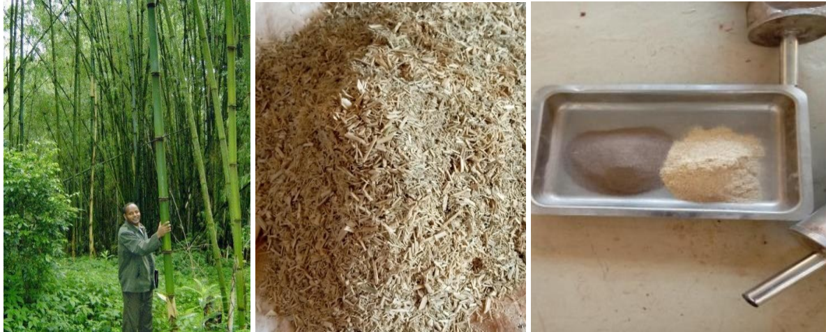
Fig. 2. Manually prepared (a) Highland bamboo tree (b) highland bamboo fiber (c) highland bamboo sawdust
