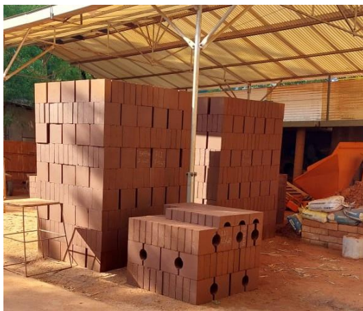
(c) CSEB blocks stacked in the production unit at Auroville Earth Institute, Pondicherry, India
