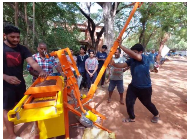
(d) Production of CSEB blocks using Auram Press 3000 machine (manually operated machine) at Auroville Earth Institute, Pondicherry, India
