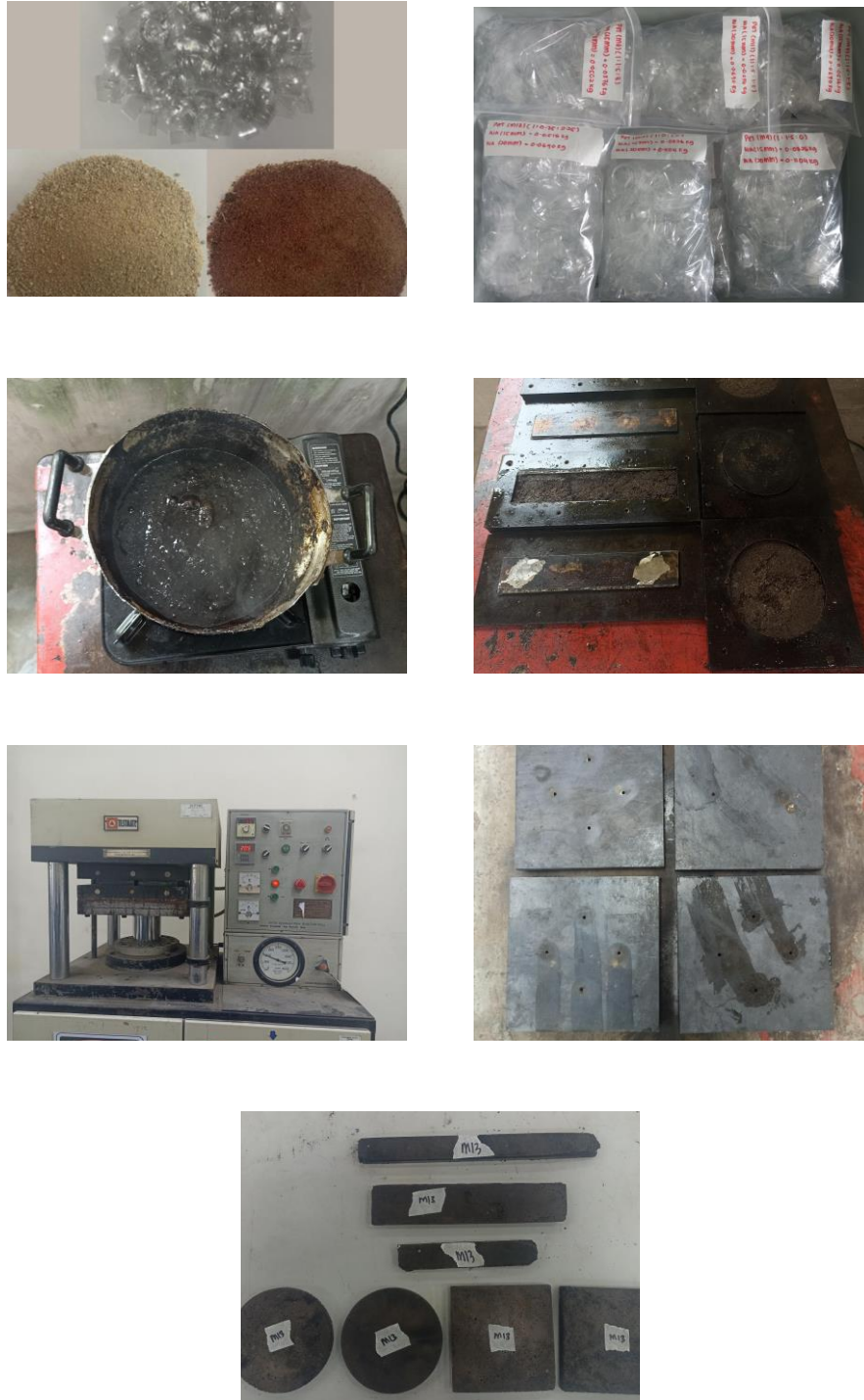
Fig 2: The fabrication process of the PET composite board
