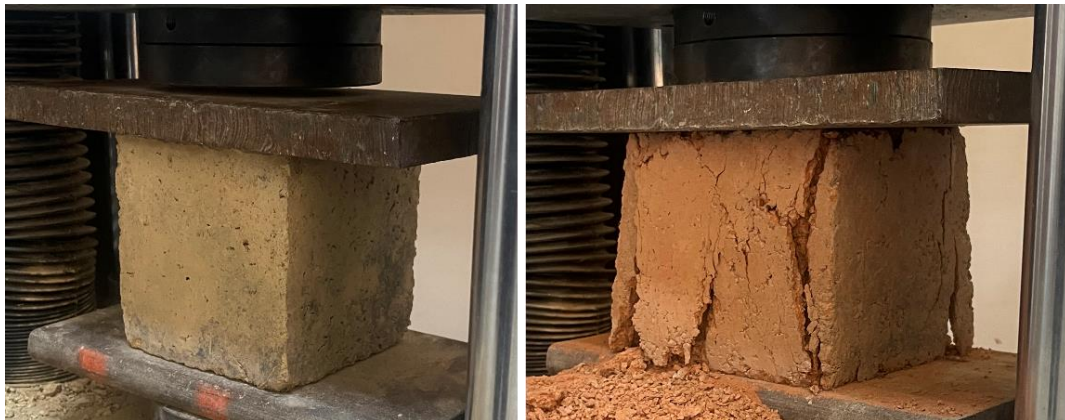
Fig. 5. Compression test setup and failure type
