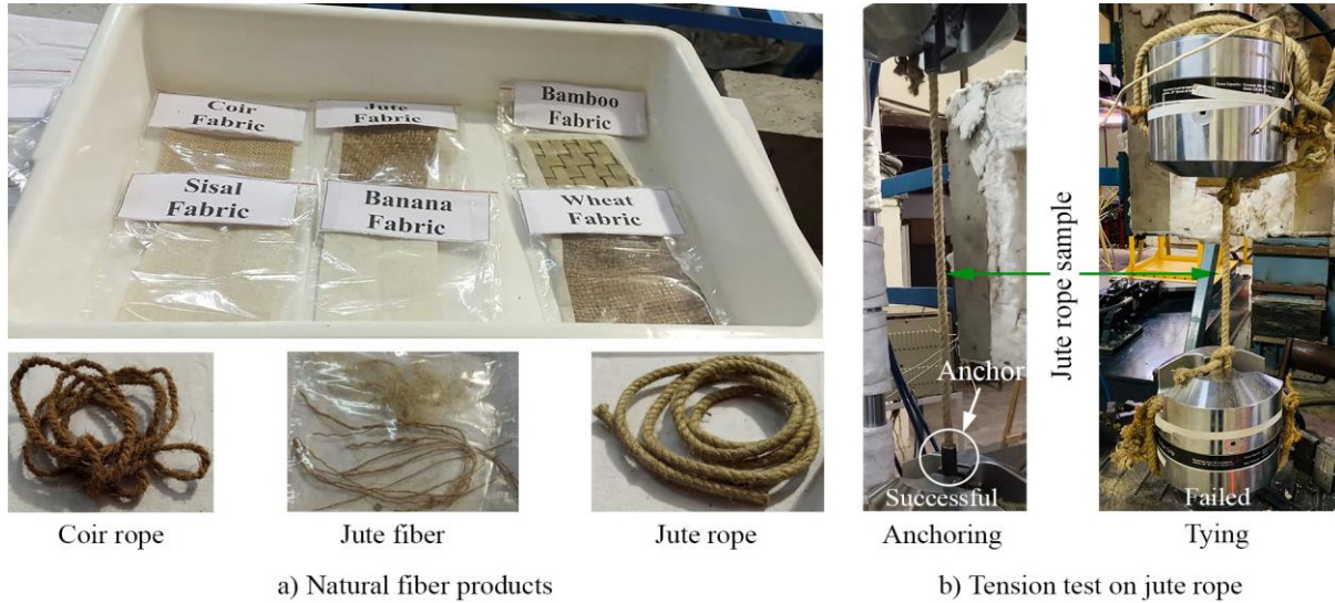
Fig. 1. a) Examples of natural fiber products; b) Tensile tests conducted on the jute ropes used in this study.
