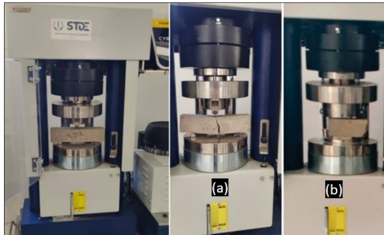
Fig. 5: STDE machine utilized to measure (a): flexural strength and (b): compressive strength.
