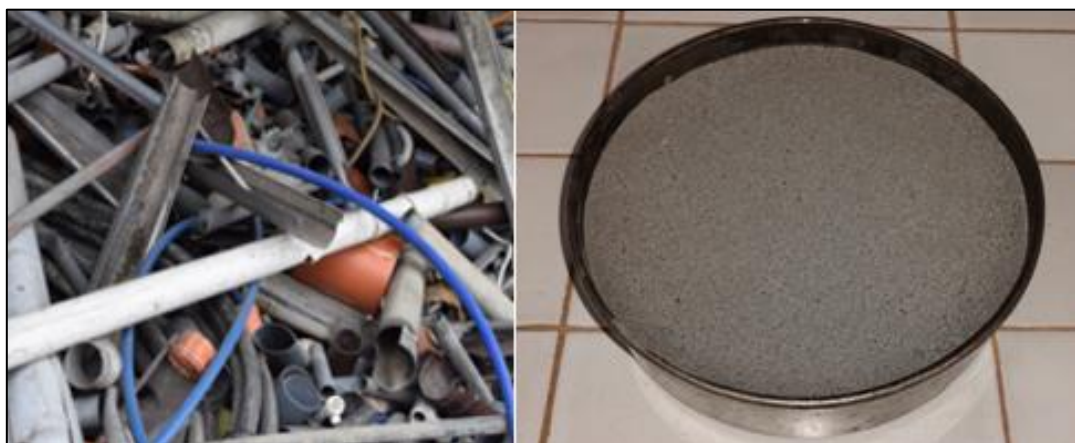
Fig. 2: Reused PVC obtained from drainage pipes
