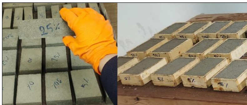
Fig. 4: Geometric configuration of the mortar specimens produced.
