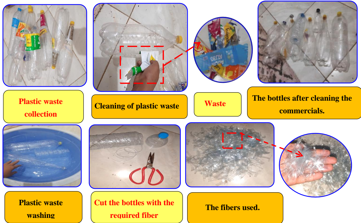
Fig. 3. The fiber manufacturing process
