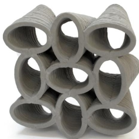
Fig. 9. 3D printed damping wall [160]
