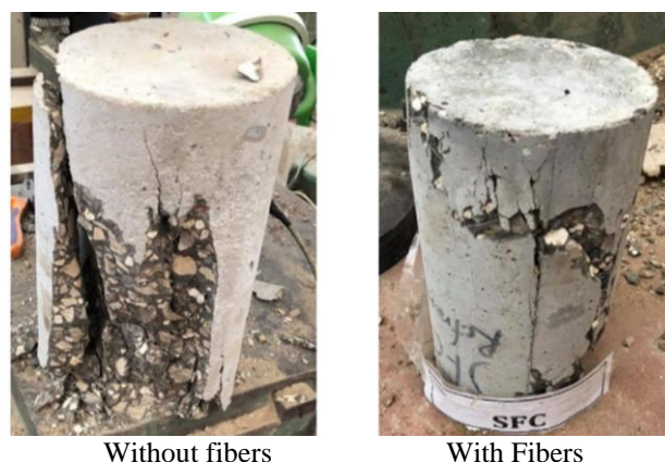
Fig. 4. Concrete failure with and without fibers [122]
