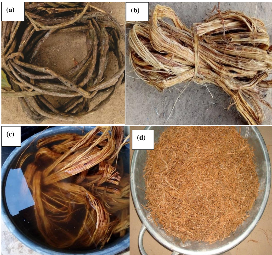
Fig. 1. Natural sponge fibre: (a) unprocessed, (b) after beating, (c) treatment, and (d) processed.
