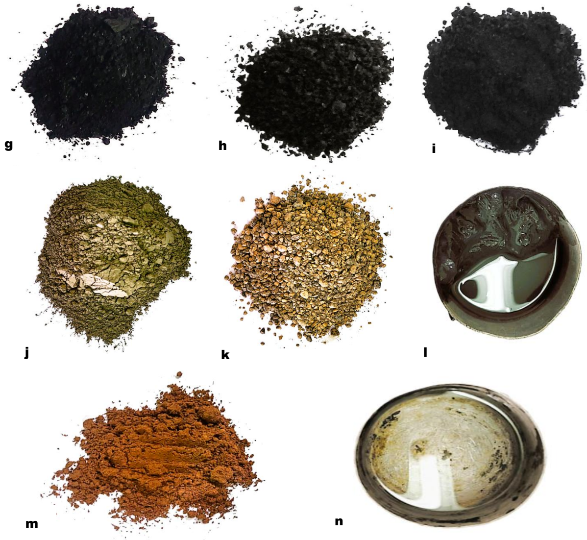
Fig. 3. Materials used in the ultra-high-strength concrete mix design: (a) Soybean Husk Ash (SHA); (b) Sugarcane Bagasse Ash (SCBA); (c) Cotton Stalk Ash (CSHA); (d) Rice Husk Ash (RHA); (e) Date Palm Fiber Ash (DPFA); (f) Pine Tree Fiber Ash (PTFA); (g) Corn Stalk Ash (CSA); (h) Peanut Shell Ash (PNSA); (i) Wheat Straw Ash (WSA); (j) Type II Portland Cement; (k) Silica Sand Fine Aggregates; (l) Calimura Nano-Silica Gel; (m) Metakaolin; (n) Water
