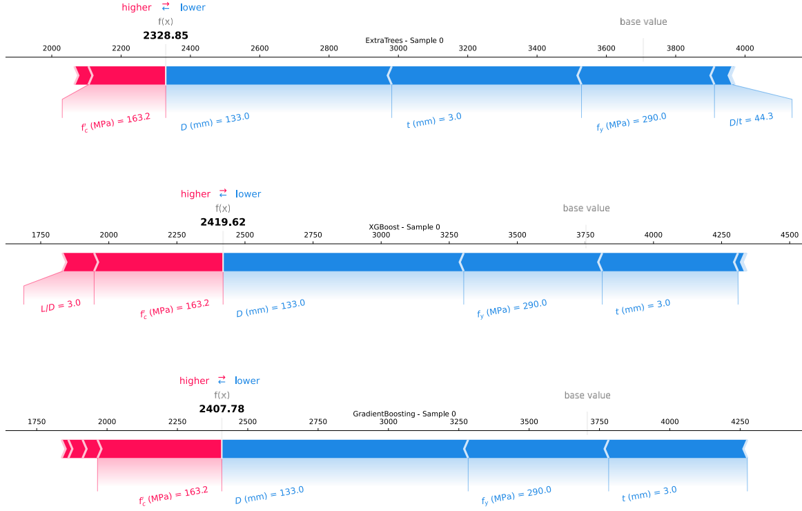
Fig. 12. SHAP force plots for individual predictions, illustrating the contribution of each feature to the final predicted axial capacity f(x) for selected samples from ML models.
