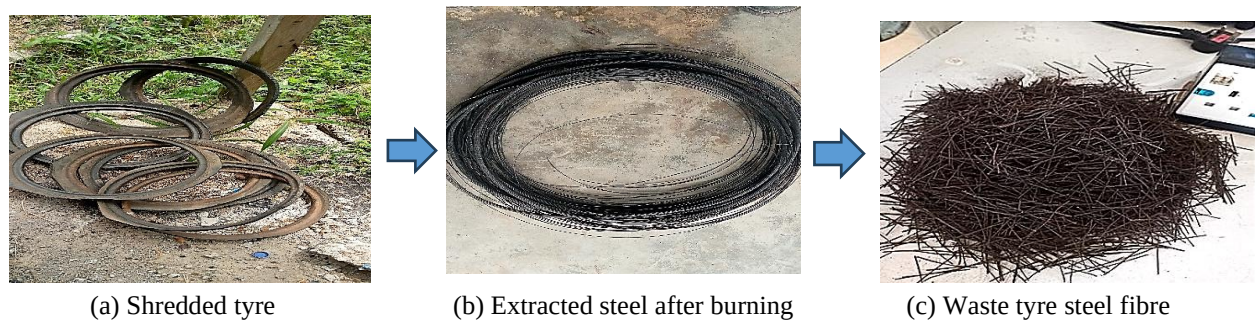
Fig. 1. Waste tyre steel fibre processing
