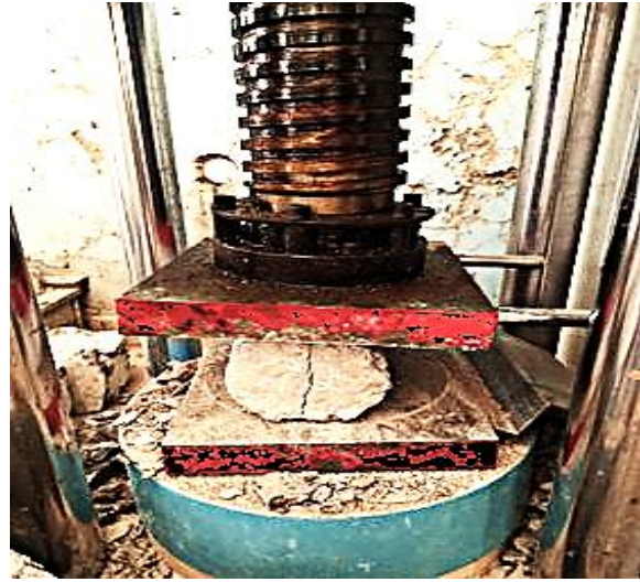
(b) Tensile strength testing
