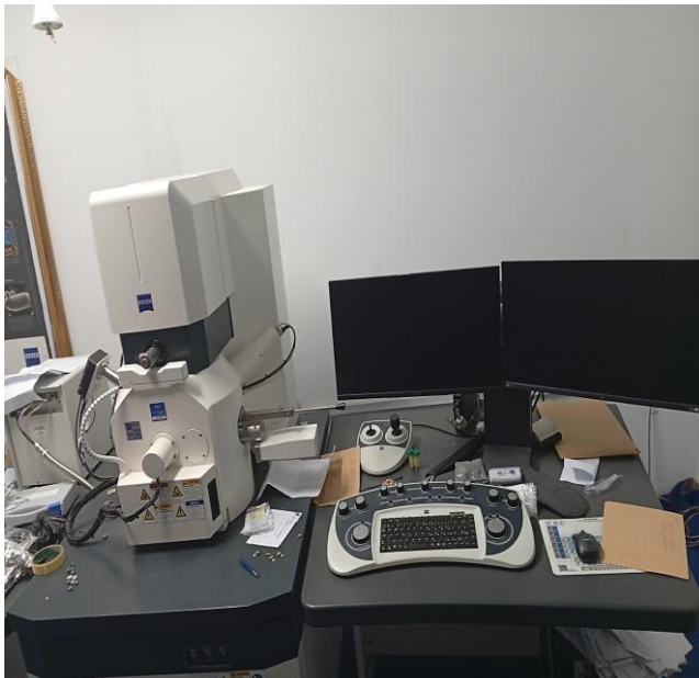
(a) SEM-EDX Machine Setup
