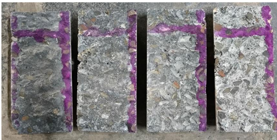
Fig. 10. Carbonation test on concrete cylinder
