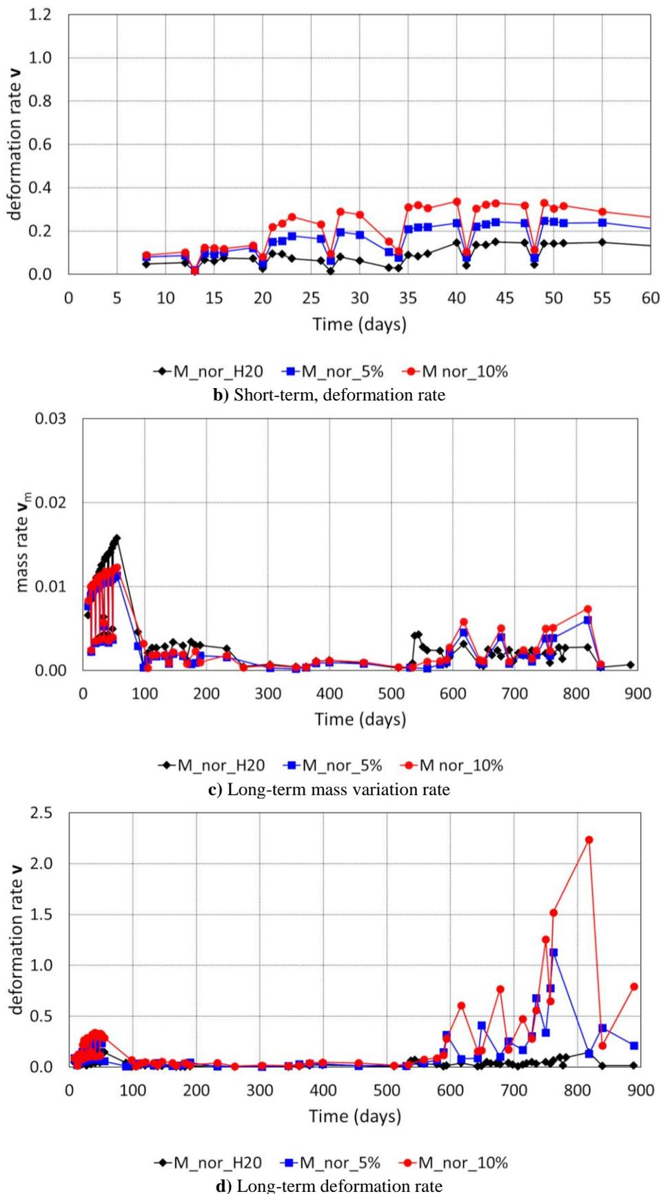
**Fig. 7.** M\_nor.: rate of deformation and mass variation over time due to three aggressive agents
