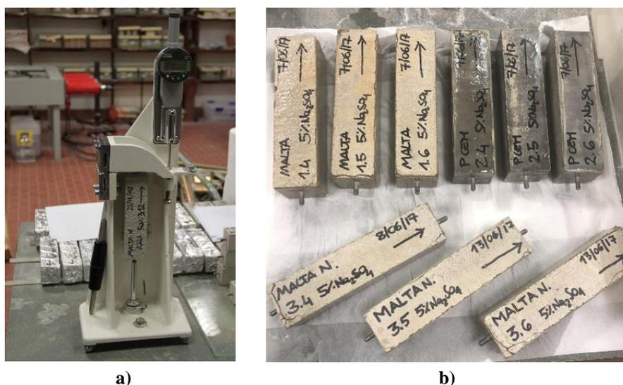
**Fig. 1.** a) Samples during the measurement phase; b) Samples during the last curing period
