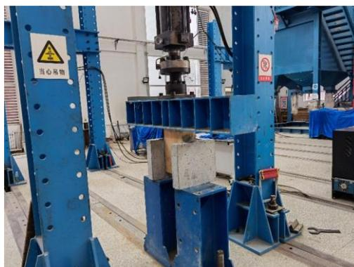
**Fig. 7.** Push-out test setup
