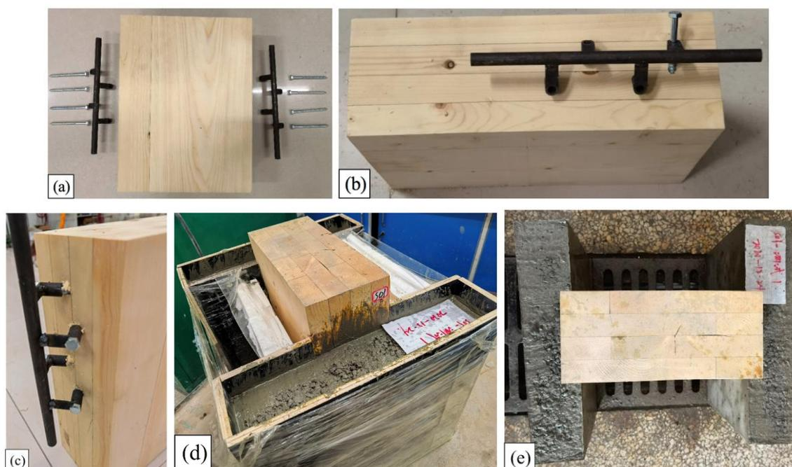
**Fig. 6.** Fabrication of a TCC connection: (a) Preparation of the components, (b) Screw driven into the hole, (c) Screws tapped into the plywood, (d) Setup of plywood formwork, and (e) Completed TCC connection
