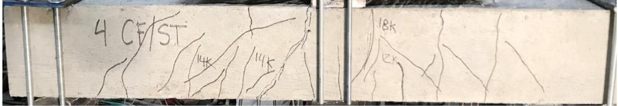
Fig. 21. Flexural failure of the hybrid (ST/CF) beam
