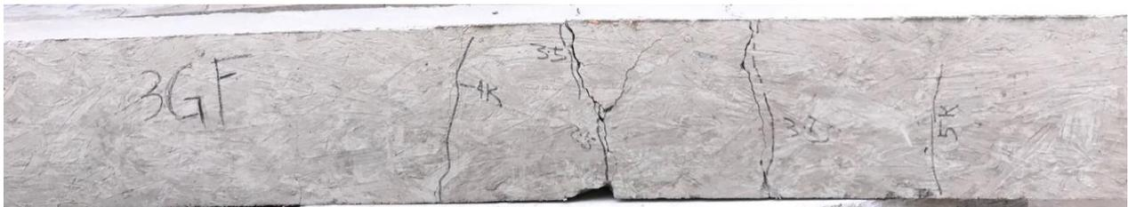
**Fig. 20.** Flexural failure of the (GF) beam
