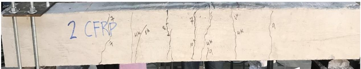
**Fig. 19.** Flexural failure of the (CF) beam
