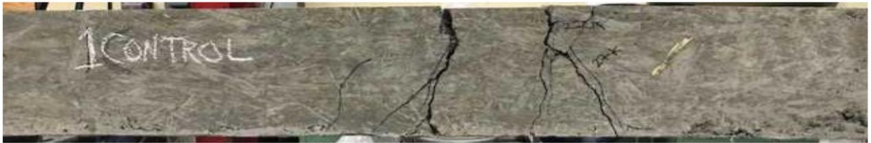
**Fig.18.** Flexural failure of the control (ST) beam
