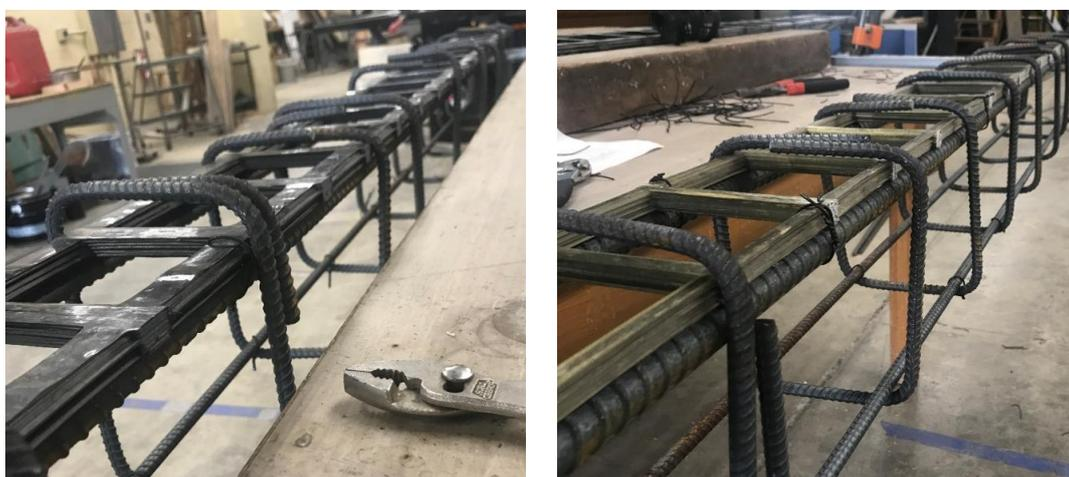
**Fig.3.** Hybrid FRP/steel reinforcement cage; a) CF/ST reinforcement, b) GF/ST reinforcement
