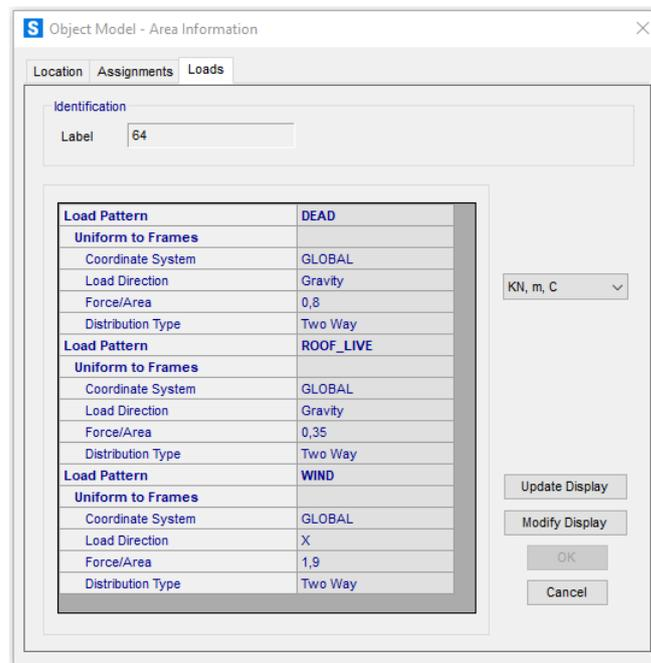
Fig. 14. Wind load applied to roof area elements.
