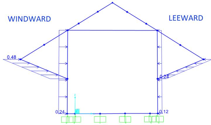
Fig. 13. Wind load applied to frame elements.
