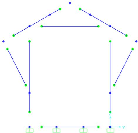
Fig. 12. Releases in frame elements (green dots).
