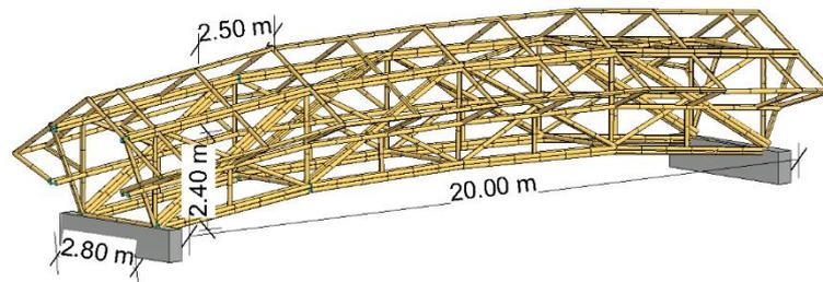
**Fig. 2.** Isometric view of the footbridge.
