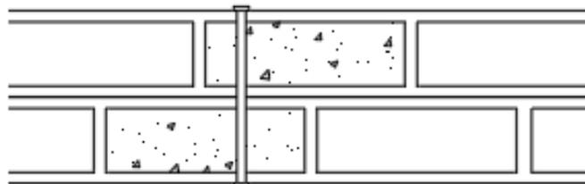
**Fig. 11.** Parallel Bolted-Mortar Infill connection.
