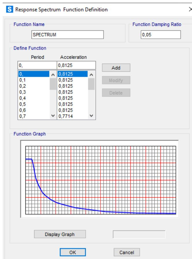
**Fig. 15.** Seismic response spectrum.
