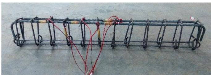
**Fig. 2.** Reinforcement cage of the beam.
