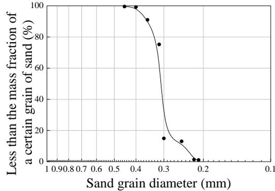
**Fig. 1.** Sand particle gradation curve.
