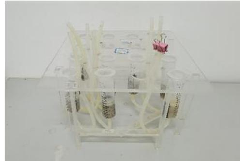
(a) Schematic diagram of the penetration test
