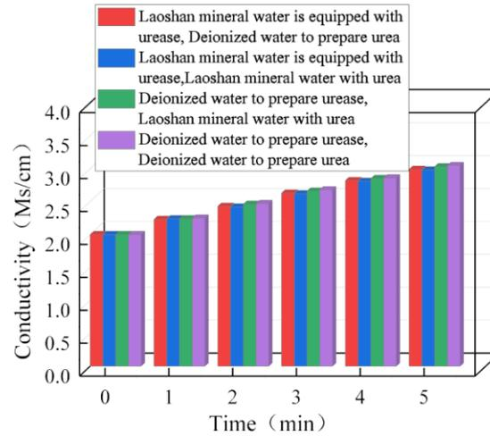
**Fig. 5.** Urease solution activity expression based on electrical conductivity.
