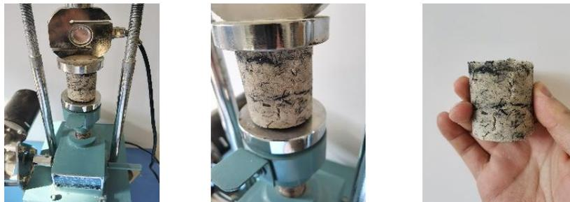
(a) Compression failure of the sample (b) The cracked sample (c) Failure surface of the sample
