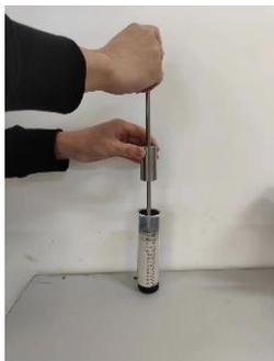
**Fig. 3.** Sample compaction.
