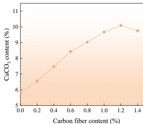
**Fig. 9.** Variation of  $\text{CaCO}_3$  content in the sand column.
