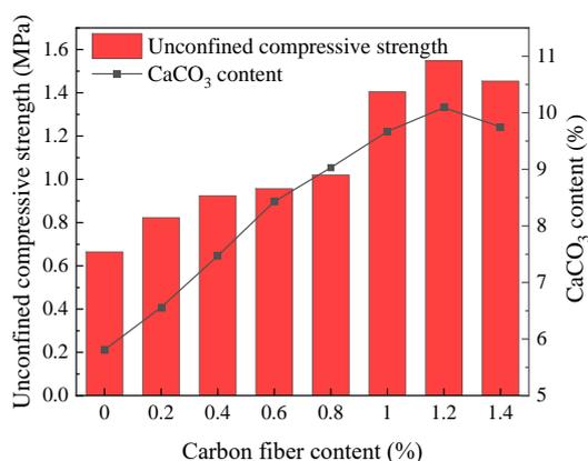
**Fig. 10.** Unconfined compressive strength of the sand column.
