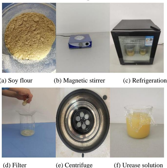
**Fig. 4.** Test Apparatus.
