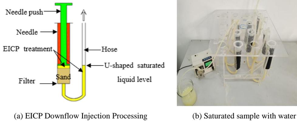
Fig. 6. EICP grouting mineralization.
