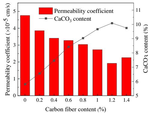
**Fig. 12.** Sand column permeability coefficient value.
