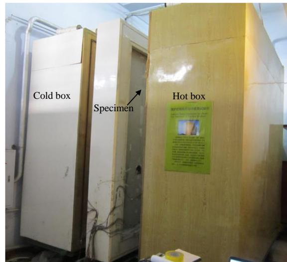
**Fig. 5.** A calibrated hot box system.
