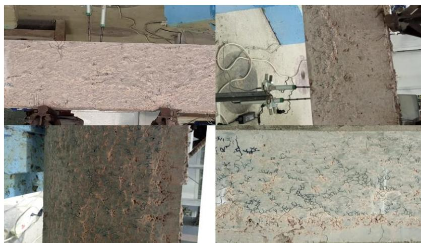
**Fig. 20.** Beams thermal cracks.
