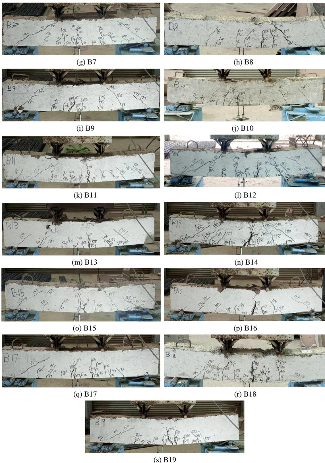
**Fig. 10.** Beams after flexural testing.
