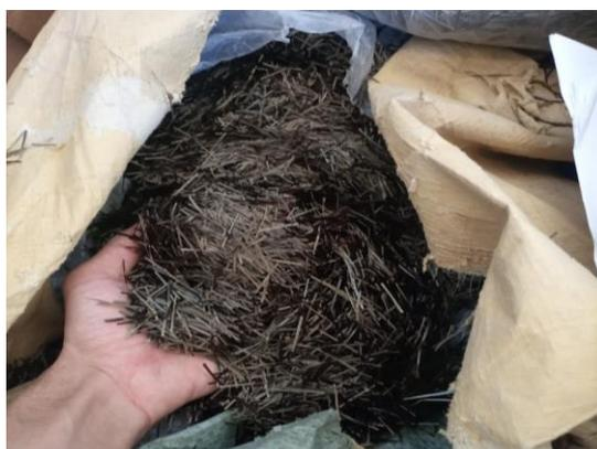
**Fig. 1.** Basalt fibers.
