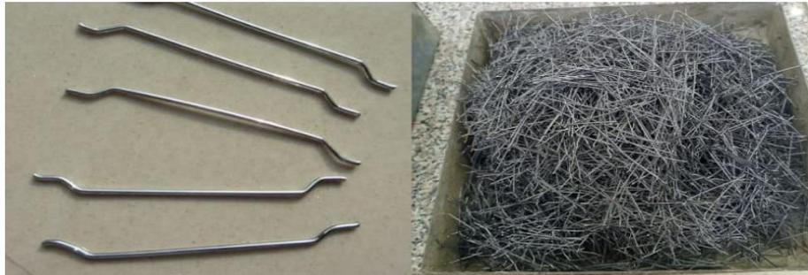
**Fig. 2.** Steel fibers.**Table 5.** Properties of steel fibers
