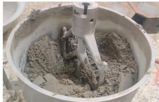
(b) Mortar mix after mixing
