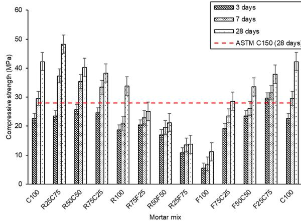
**Fig. 10.** Compressive Strength Test Results of Mortar Mixes.
