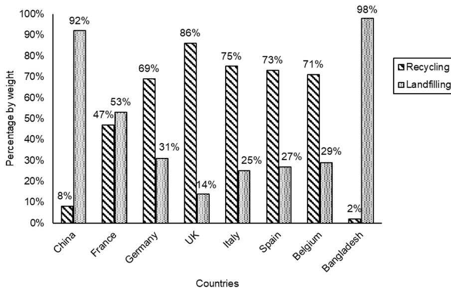
**Fig. 2.** Landfilling and recycling status of CDW in different countries [21].
