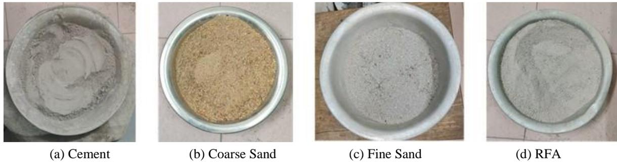
**Fig. 3.** Materials used to prepare mortar mixes.
