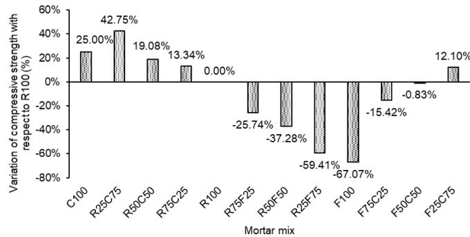
**Fig. 11.** Variation in Compressive Strength in percentage with respect to 100% recycled fine aggregate mortar.
