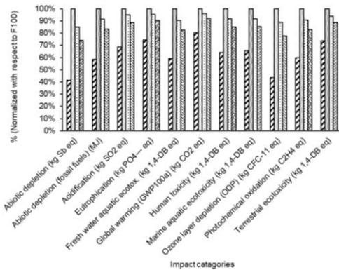
**Fig. 14.** Environmental impact of cement mortars (CML-IA baseline method)
