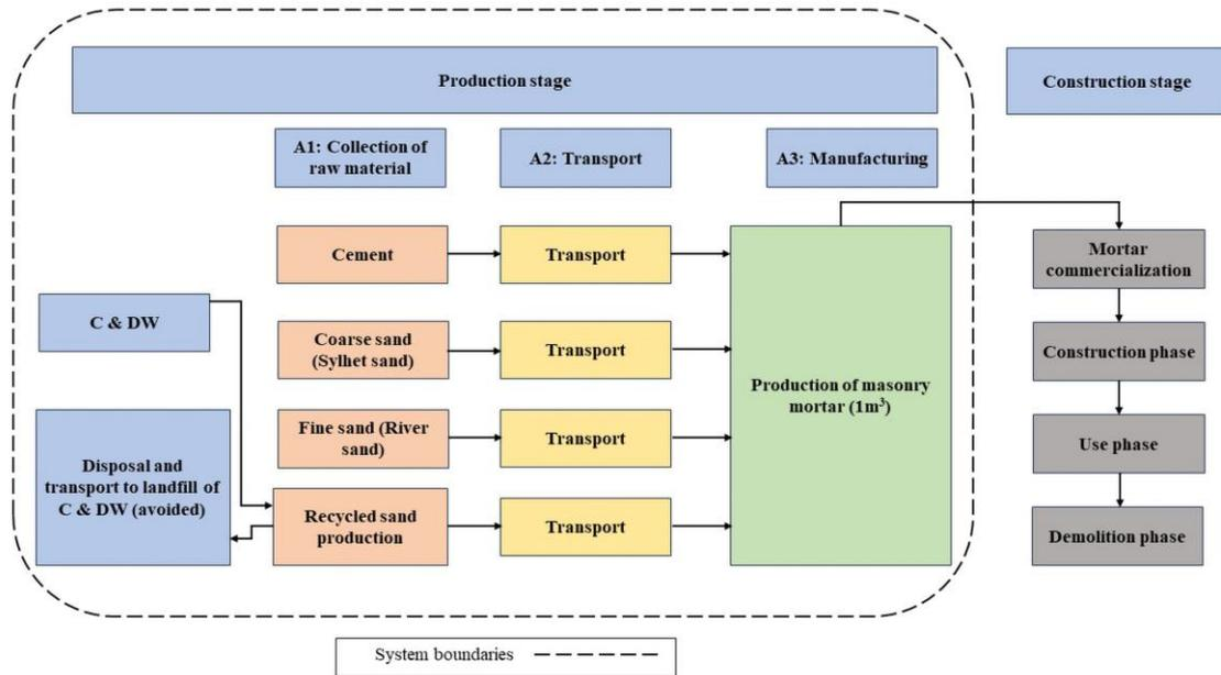
Fig. 5. System boundary of cement mortar.
