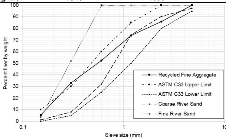
**Fig. 8.** Gradation curve of the fine aggregates.
