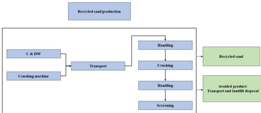
Fig. 6. Production process of recycled fine aggregate.
