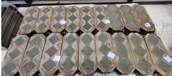
(c) Mortar mix in the molds
