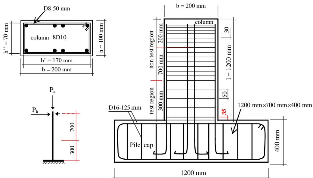
**Fig. 1.** Column without AAC.
