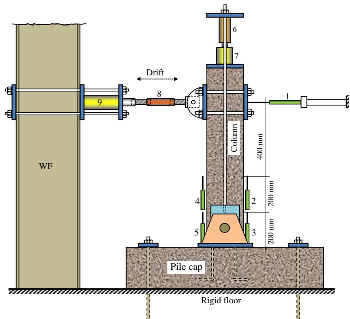
**Fig. 7.** Schematic test setup [44-46] adapted to the laboratory conditions, 1-5 = LVDT (linear variable displacement transducer), 6 = single-acting hydraulic jack, 7 = single-acting load cell, 8 = double-acting load cell, 9 = double-acting hydraulic jack, = quasi-cyclic load direction.
