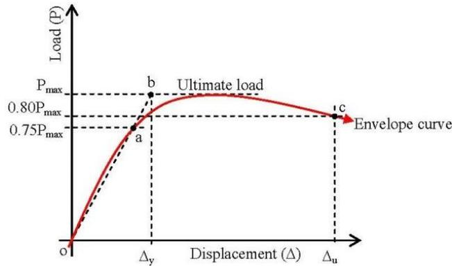
**Fig. 5.** Definition of yield displacement [40,41].
