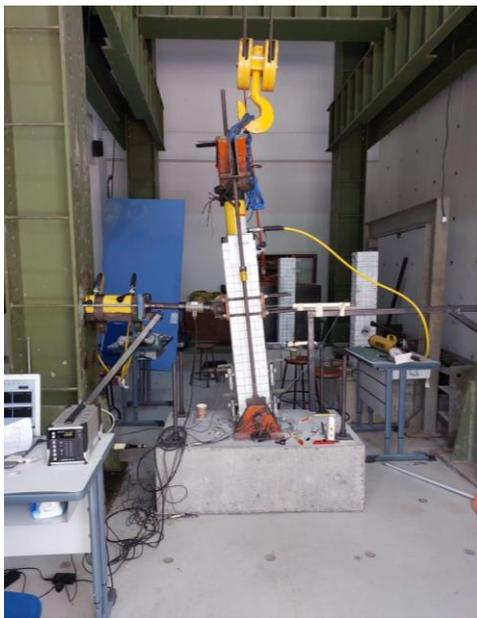
**Fig. 6.** Actual test setup and drift that occurred during testing.
