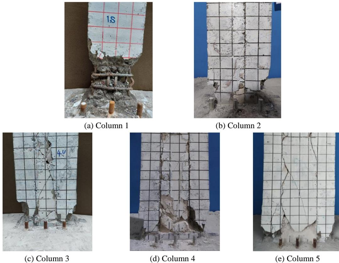
**Fig. 10.** Column cracks and plastic hinges occurred in the range of 100 to 150 mm.
