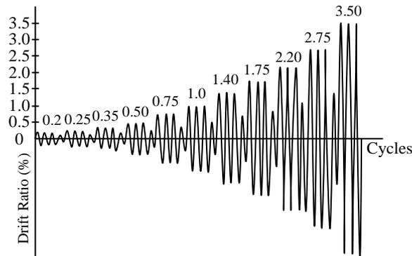
**Fig. 3.** Displacement controlled cycles [38].
