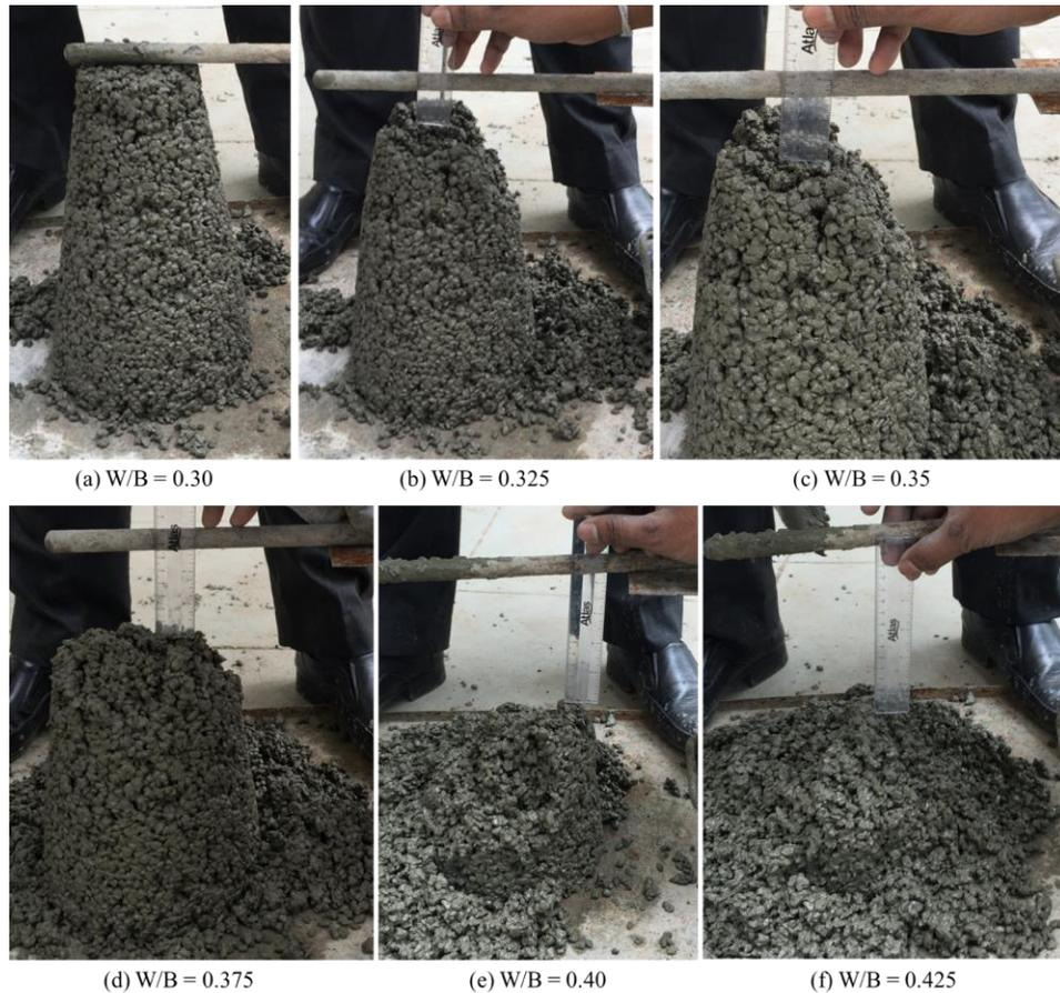
**Fig. 2.** Slump variation with  $W/B$  ratio.
