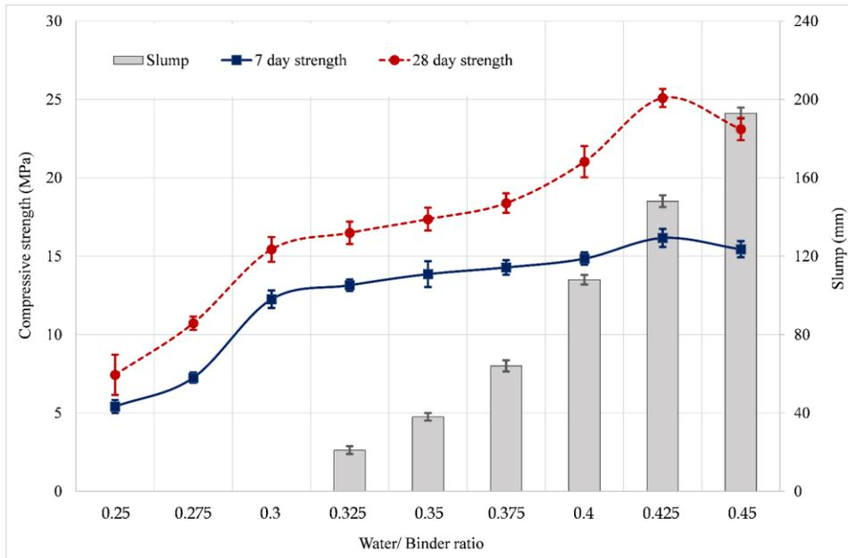
Fig. 4. Compressive strength variation with  $W/B$  ratio.
