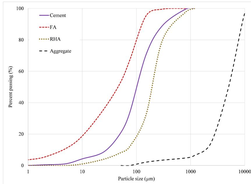
**Fig. 1.** Particle size distribution of the materials.
