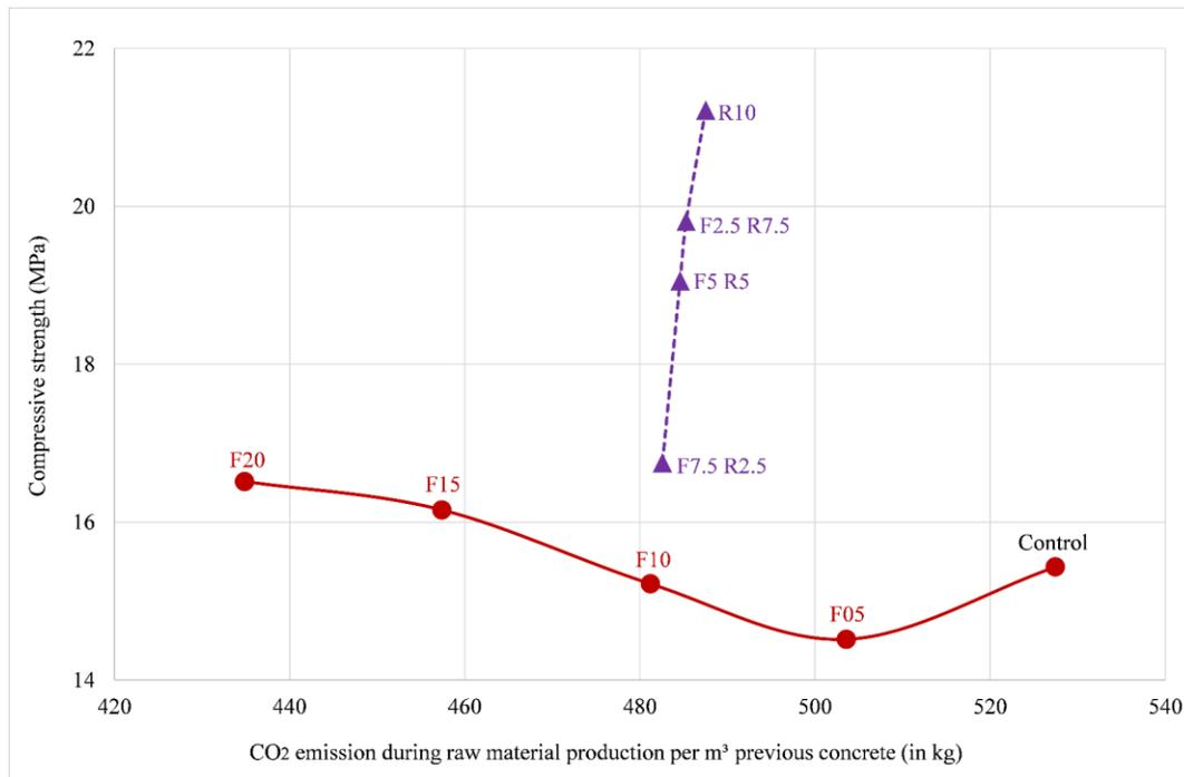
**Fig. 9.** CO<sub>2</sub> emission analysis of raw material used for pervious concrete with various mix ratios.
