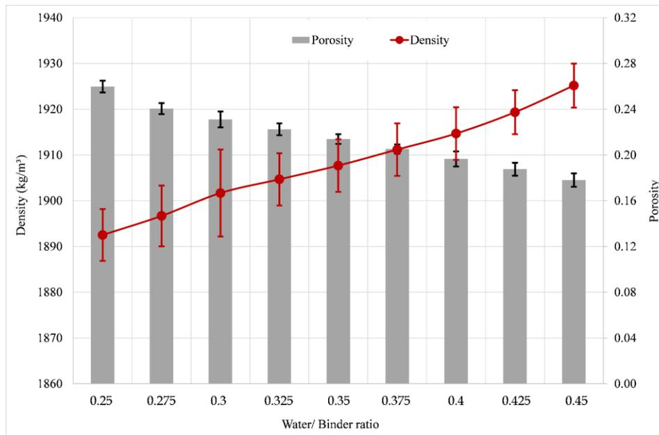
**Fig. 3.** Density and porosity variation with  $W/B$  ratio.
